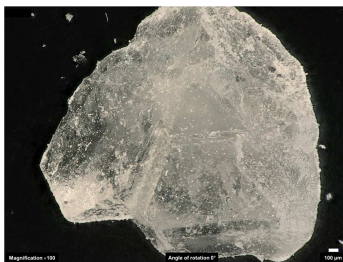
Figure 1. Digital microscope observation of one of our millimeter-scale borate crystals recovered after hydrolysis of AB in alkaline conditions: magnification \times 100 ; angle of rotation 0^\circ ; scale bar 100\ \mu\text{m} .
