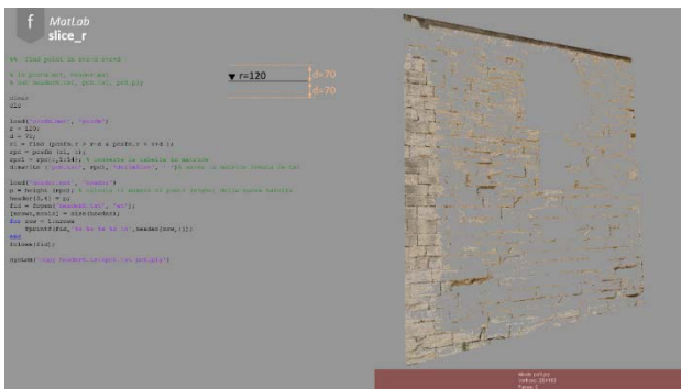
Figure 17. Selection of point cloud, starting from a given value of r (red) and a selectable range.
