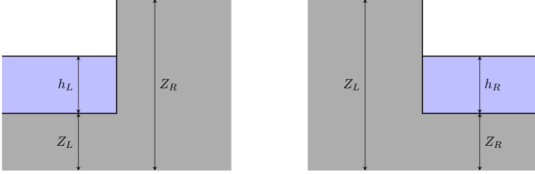
Figure 3: Physical lake at rest configurations not governed by (1.7). Left panel: lake at rest with h_R = 0 and h_L + Z_L \leq Z_R . Right panel: lake at rest with h_L = 0 and h_R + Z_R \leq Z_L .
