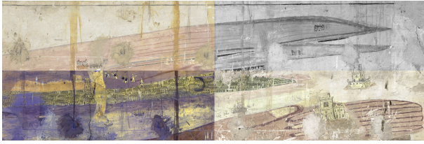
Figure 9: Example of ad-hoc multispectral photogrammetric acquisition ; registered orthophotomosaic in visible (top-left), infrared (top-right), ultraviolet fluorescence (bottom-left) and mean composite picture (bottom-right) on Anamorphosis case-study.
