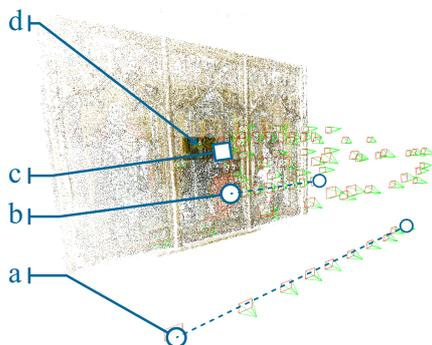
**Figure 3:** Multidimensional blocks merged : global (a) and close-up (b) photogrammetry, multistereo H-RTI (c) and multitemporal/multispectral Technical Photography (d) on Venasque case-study.
