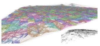
Fig. 5: Result of the proposed approach on 1.98 billion of points  $6km^2$  with 2cm spatial resolution. This figure shows the whole scene. Only finalized cells during the last step are shown. Triangles of the same tile have the same color.
