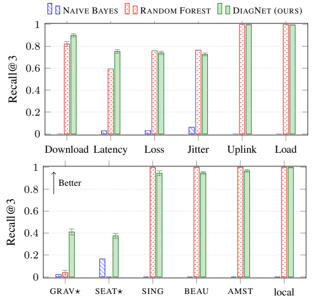
Fig. 6. Detail of models recalls per fault family (top) and fault region (bottom). Regions hidden during training are indicated with a star *. Again, RANDOM FOREST gives best results for known landmarks, but DIAGNET is the only solution able to adapt to the different scenarios, with optimal results for local faults.
