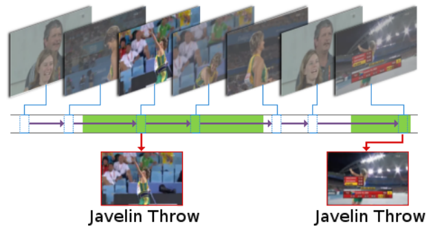
Fig. 1: Overview of the proposed spot frame extraction framework. It extracts one spot frame per action occurrence (in green in the figure) by sparsely browsing the video.
