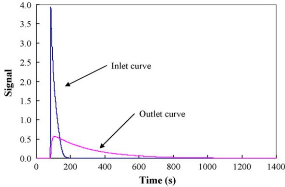
Fig. 2. Typical response of the conductimetric method: inlet and outlet signals ( $N = 1500$  rpm,  $Q = 1200$  ml h<sup>-1</sup>).
