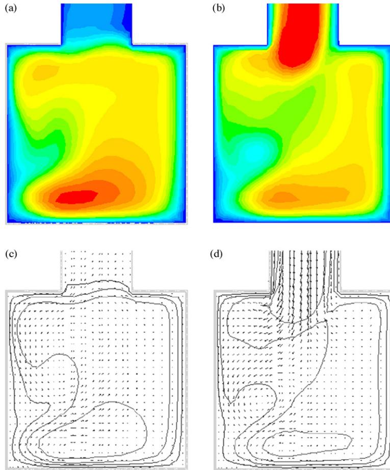
Fig. 13. Modification of the flow structure due to the feeding injection. Velocity contours inside the reactor for (a) 200 rpm,  $180 \text{ ml h}^{-1}$ , (b) 200 rpm,  $7200 \text{ ml h}^{-1}$ . Velocity vectors showing the flow disturbance (c) 200 rpm,  $180 \text{ ml h}^{-1}$ , (d) 200 rpm,  $7200 \text{ ml h}^{-1}$ .
