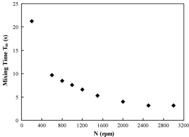
Fig. 9. Mixing time numerical prediction: evolution of the mixing time with the impeller rotation velocity.
