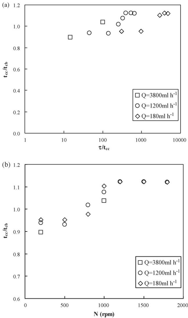
Fig. 12. (a) Comparison of the mean circulation time in continuous and batch conditions as a function of the  $\tau/t_{cc}$  ratio for different flowrates. (b) Comparison of the mean circulation time in continuous and batch conditions as a function of the impeller rotation speed for different flowrates.
