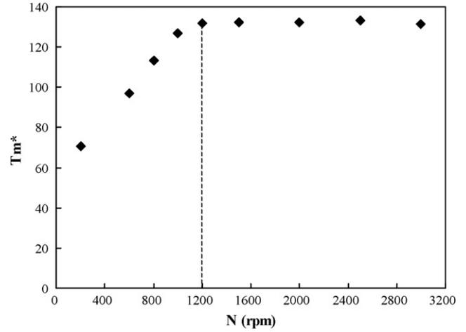
Fig. 10. Mixing time numerical prediction: dimensionless mixing time.
