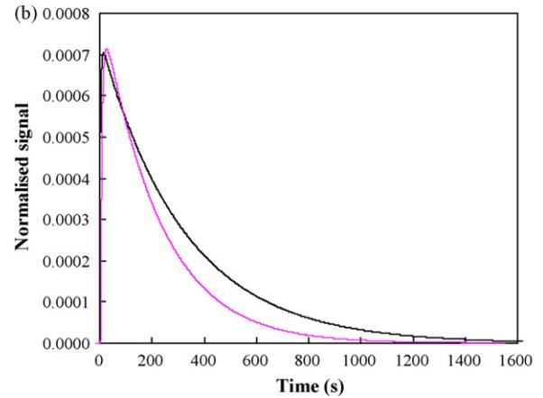
Fig. 6. (a) Experimental and simulated values of the mean residence time. (b) Experimental and numerical prediction of the residence time distribution.
