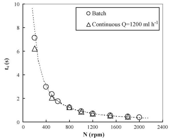
Fig. 11. Mean circulation times obtained for batch and continuous conditions for different impeller rotation speeds and for a flowrate of 1200 ml h<sup>-1</sup>.
