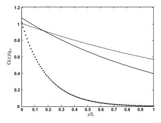
**Fig. 4.** Example of light attenuation profiles (solid line: t = 0 h, X = 0.04 kg m<sup>-3</sup> – dotted line: t = 111 h, X = 0.37 kg m<sup>-3</sup> – dashed line: same as dotted line, but assuming no pigments degradation, see text for details).
