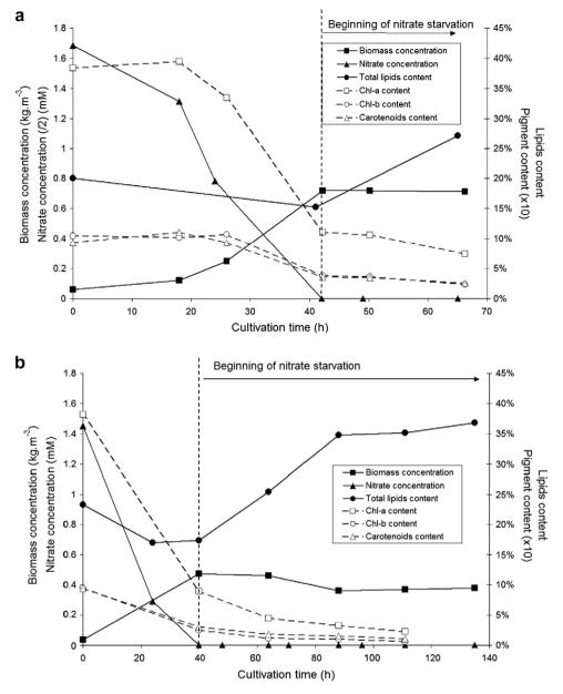
Fig. 3. Time course profiles during progressive nitrate starvation with No = 3.37 M (a) and No = 1.45 M (b) (batch culture, qo = 270 µmole m<sup>-2</sup> s<sup>-1</sup>).
