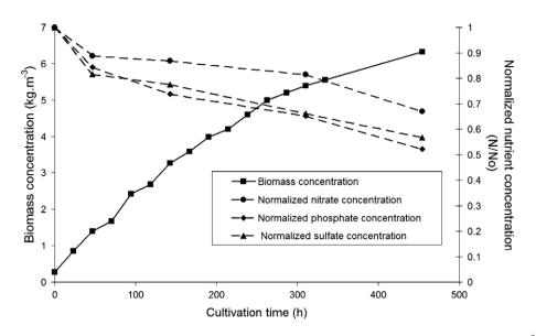
Fig. 1. Time course of biomass and macronutrients concentrations (light-limited growth, batch culture,  $q_0 = 270 \,\mu\text{mole m}^{-2} \,\text{s}^{-1}$ ).
