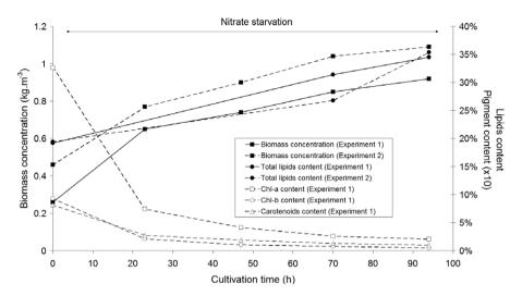
**Fig. 5.** Time course profiles during sudden nitrate starvation with initial biomass concentration  $X_0 = 0.26$  kg m<sup>-3</sup> (Experiment 1) and  $X_0 = 0.46$  kg m<sup>-3</sup> (Experiment 2) (batch culture,  $q_0 = 270$  µmole m<sup>-2</sup> s<sup>-1</sup>).
