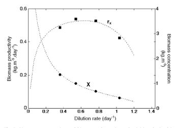
**Fig. 2.** Biomass concentration and biomass volumetric productivities obtained in continuous mode (light-limited growth,  $q_o = 270 \ \mu \text{mole m}^{-2} \ \text{s}^{-1}$ ).
