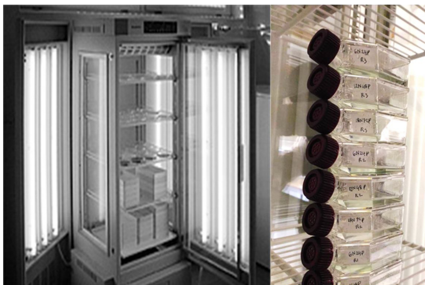
Fig. 1. Culture chamber SANYO MLR-350 (left) and culture flask positions inside the culture chamber (right).
