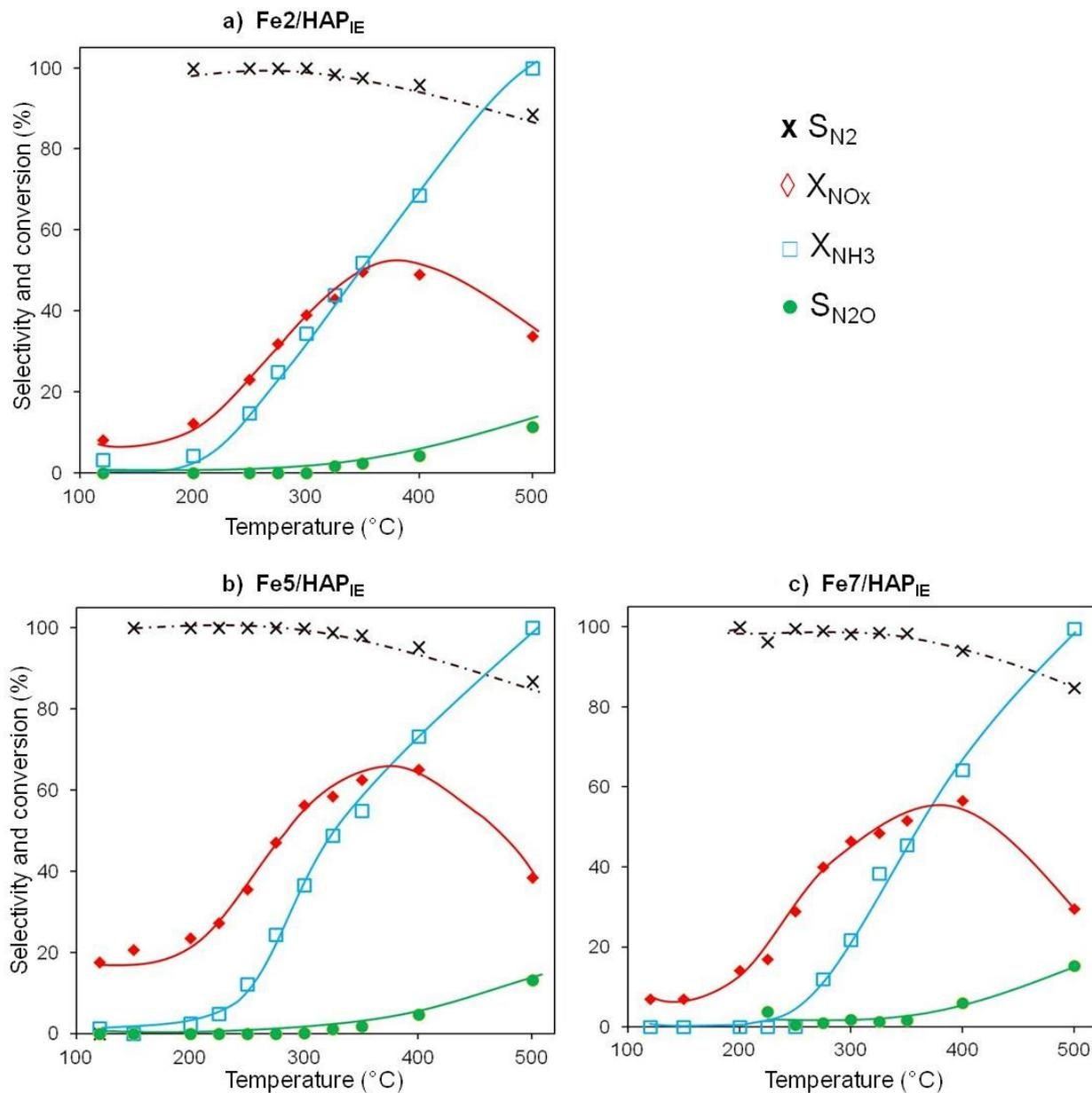
**Fig. 2.**  $\text{NH}_3$ -SCR catalytic results on Fe/HAP samples prepared by *flash* ionic exchange (a-c): profiles of conversion of the fed species ( $\text{NO}_x$  and  $\text{NH}_3$ ) and selectivity of formed species ( $\text{N}_2$  and  $\text{N}_2\text{O}$ ) as a function of reaction temperature with the use of  $\text{NH}_3/\text{NO}$  ratio equal to one.
