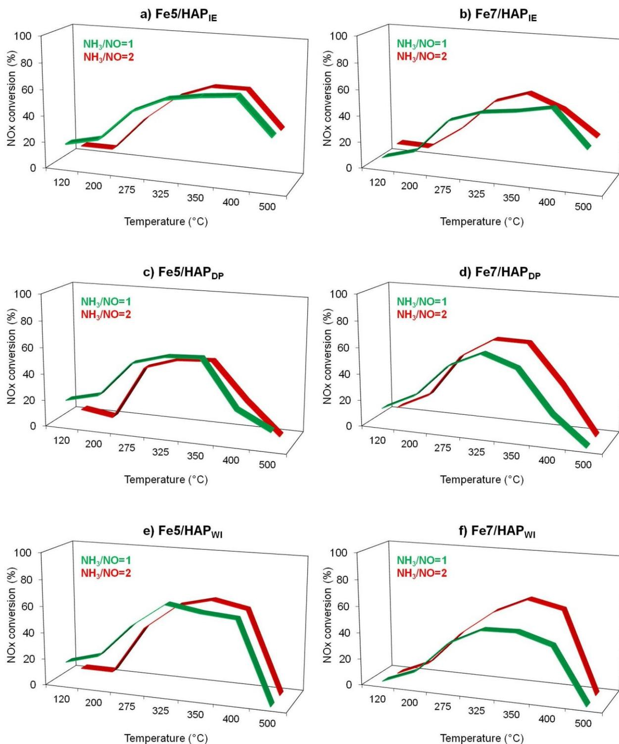
**Fig. 4.** NH<sub>3</sub>-SCR catalytic results on Fe/HAP samples prepared by *flash* ionic exchange (a-b), deposition-precipitation (c-d) and incipient wetness impregnation (e-f): comparison of NO<sub>x</sub> conversion as a function of reaction temperature at different ammonia concentrations (NH<sub>3</sub>/NO=1, green and NH<sub>3</sub>/NO=2, red).
