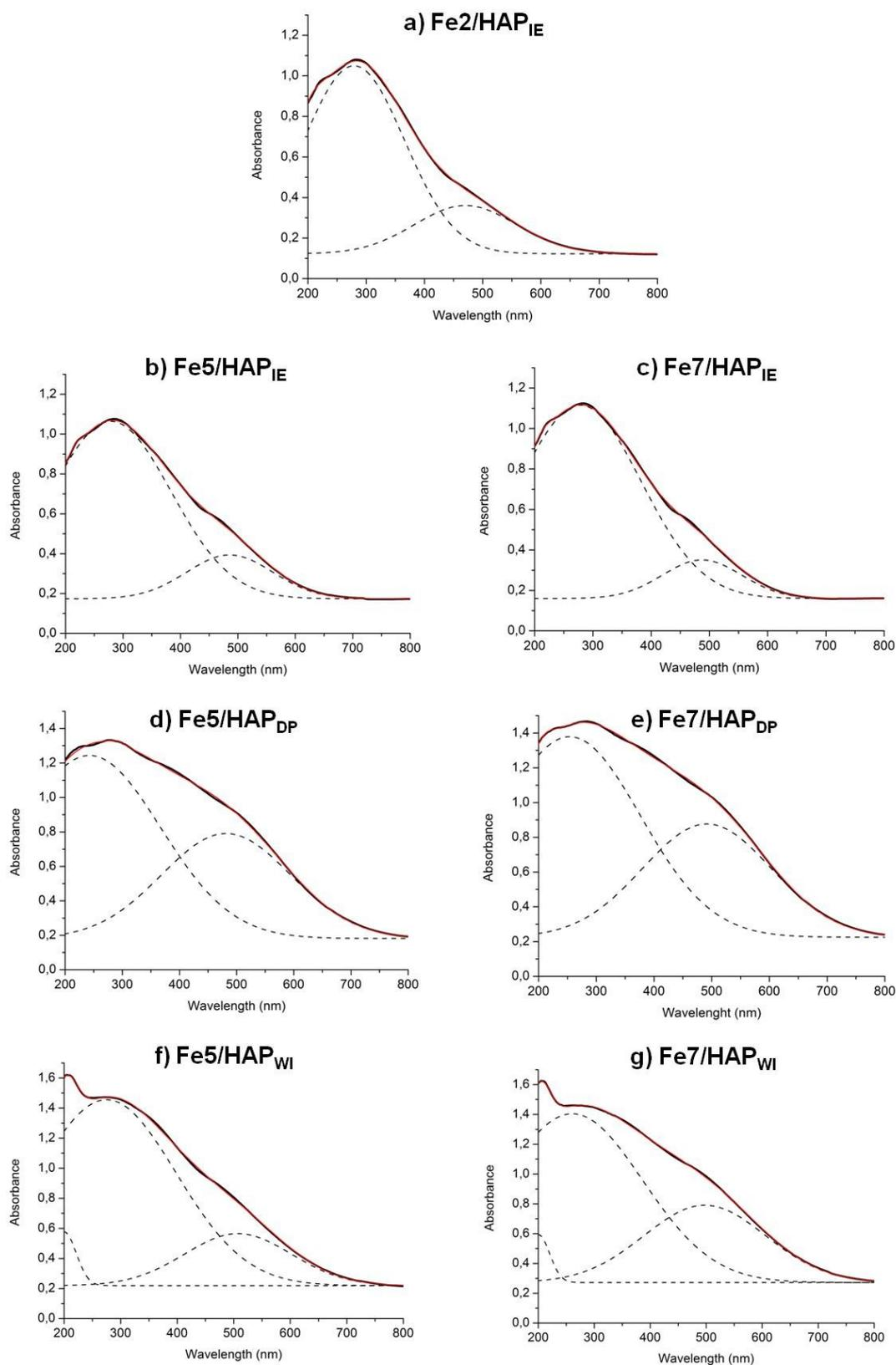
**Fig. 6.** UV-Vis-DR spectra (black curves) of Fe/HAP samples prepared by *flash* ionic exchange (a-c), deposition-precipitation (d-e) and incipient wetness impregnation (f-g). Total calculated curves (red lines) and decomposed curves (dotted black lines) are also reported..
