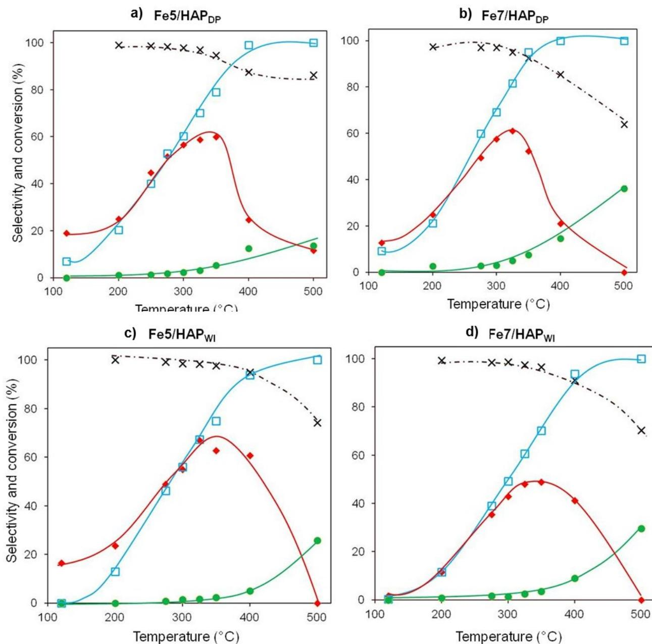
**Fig. 3.** NH<sub>3</sub>-SCR catalytic results on Fe/HAP samples prepared by deposition-precipitation (a-b) and incipient wetness impregnation (c-d): profiles of conversion of the fed species (NO<sub>x</sub> and NH<sub>3</sub>) and selectivity of formed species (N<sub>2</sub> and N<sub>2</sub>O) as a function of reaction temperature with the use of NH<sub>3</sub>/NO ratio equal to one.
