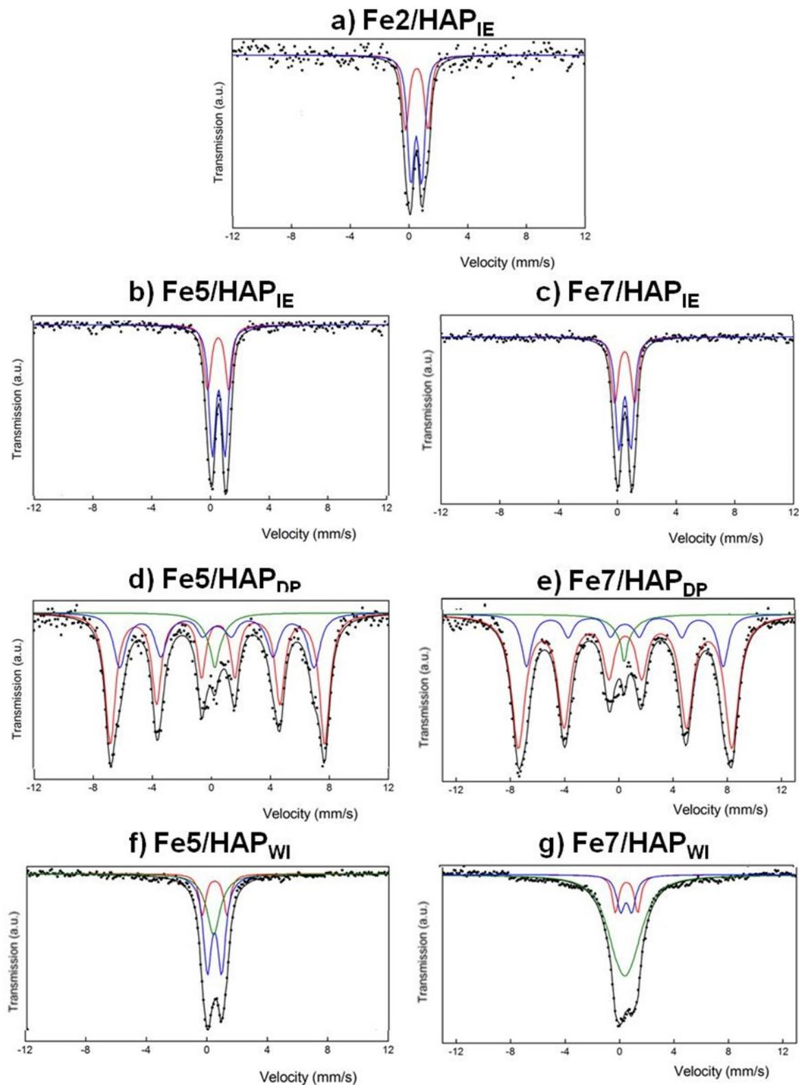
**Fig. 5.** Mössbauer spectra of Fe/HAP samples prepared by *flash* ionic exchange (a-c), deposition-precipitation (d-e) and incipient wetness impregnation (f-g) at  $-260.15^{\circ}\text{C}$  (13 K). Black points are the experimental values; green, red, and blue lines are interactions obtained from fitting and assigned; and black lines are the convolution of all the interactions.
