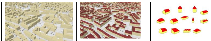
Figure 2 Buildings from Bavaria: LOD1 (left); LOD2 (middle); 13 standard roof shapes from ALKIS®-Objectcatalog for LOD2 Buildings (right)
