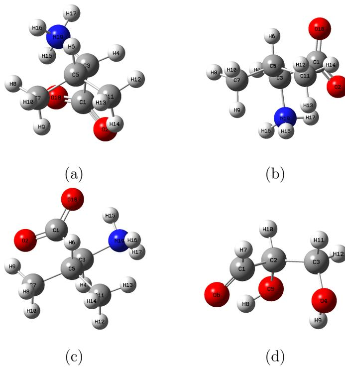
Figure 1: Three Optimized structures of the L-Valine zwitterion and the lowest energy geometry of D-glyceraldehyde. (a) *Trans/Gauche+*; (b) *Gauche+/Gauche-*; (c) *Gauche-/Trans*; (d) D-glyceraldehyde
