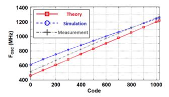
Figure 13: Comparison between the measured, the simulated (post-layout) and the theoretical DCO transfer characteristic, for  $V_{DD} = 1.1 \text{ V}$ .
