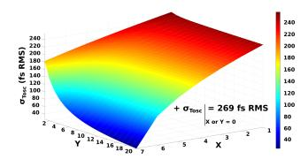
Figure 6: DCO period jitter predicted with equation (24).
