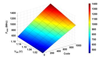
Figure 14: 3D graphic of Circuit-M oscillation frequency tuned by the input code and the supply voltage  $V_{DD}$ .
