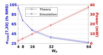
Figure 8: Illustration of the power-jitter trade-off related to  $W_{seP}$  for all tuning cells enabled.
