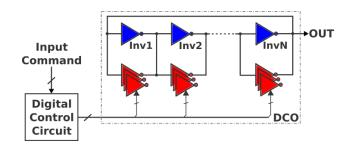
Figure 1: Architecture of the tri-state inverter based DCO.
