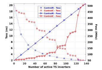
Figure 10: DCO Period and frequency responses, as a function of the number of active tuning cells, and for  $Control_R$  and  $Control_C$ .
