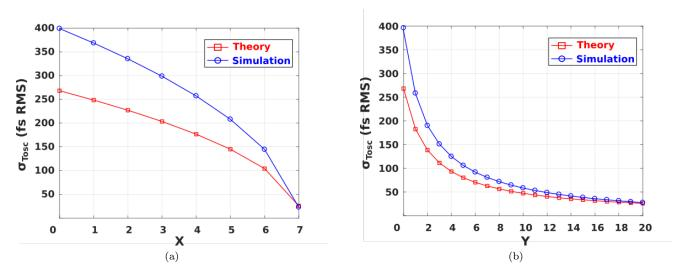
Figure 7: For  $W_{seP}=64~\mu m$ : a) - Jitter as a function of  $\mathcal{X}$  for  $\mathcal{Y}=Q=20$ ; b) - Jitter as a function of  $\mathcal{Y}$  for  $\mathcal{X}=N=7$ .
