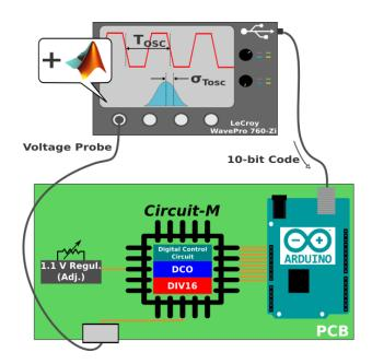
Figure 12: Experimental setup for the characterization of *Circuit-M*.
