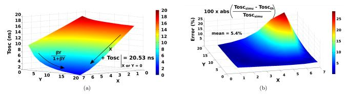
Figure 5: For  $W_{seP}$ =64  $\mu$ m: (a) - Simulation result of the oscillation period as a function of the bi-dimensional command; (b) - Absolute error between theory and simulation.
