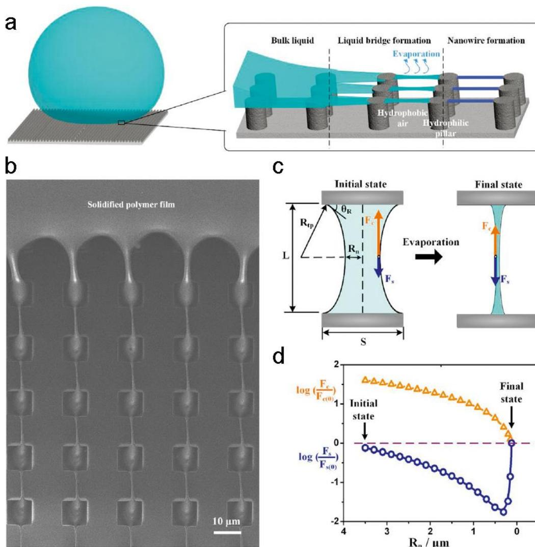
**Fig. 8** (a) Schematic illustration and (b) SEM image of the formation process of oriented NWs during the regular liquid rupture upon a superhydrophobic pillar-structured substrate. (c) Schematic illustration of  $F_c$  and  $F_s$  inside one liquid bridge. (d) Dependence of  $F_c$  and  $F_s$  on the radius of the liquid bridge neck ( $R_n$ ). The two forces get equal to each other as water is evaporated. Reproduced with permission from ref. 115. Copyright 2019 Elsevier Inc.
