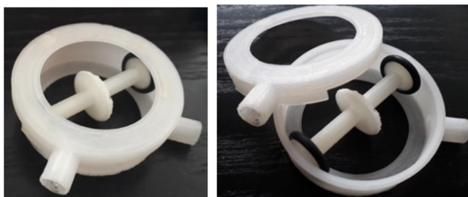
Figure 14: A bisector machine using rubber wheels to avoid gears. The two rubber wheels share the same axis, but they can rotate independently.
