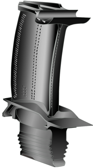
Figure 1: Schematic of a high-pressure turbine blade [1]. Internal cooling channels allow the cool air to exit and protect the outer surface of the blade with a cooling film.
