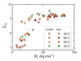
Fig. 17. Elongation at break as a function of  $M_{\rm n}$  for both TPUs, at four ageing temperatures.
