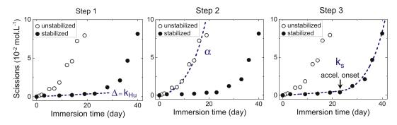
Fig. 12. Model constants determination by curve fitting of experimental scissions (ageing at 80 °C).
