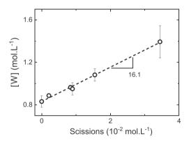
Fig. 11. Water concentration [W] change with scissions (unstabilized TPU during immersion at 80  $^{\circ}\text{C}\text{)}.$
