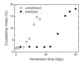
Fig. 8. Crystallinity Index determined by WAXS as a function of immersion time for both TPUs aged in water at 80  $^\circ$ C.
