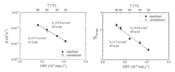
Fig. 3. Diffusion coefficient D and mass uptake at saturation %m sat. at different temperatures, for stabilized and unstabilized TPUs.
