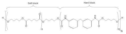
Fig. 1. Ester-based TPU chemical structure.
