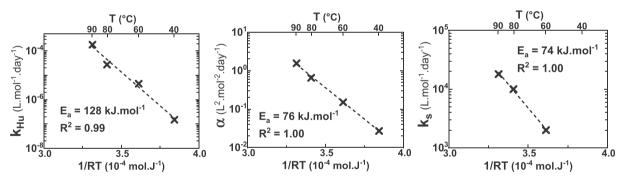
Fig. 16. Temperature dependence of uncatalysed hydrolysis rate constant k<sub>Hu</sub>, catalysis constant  $\alpha$  and stabilization reaction rate constant k<sub>s</sub>.
