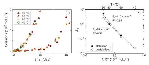
Fig. 14. (a) Time-temperature superposition of chains scissions, for unstabilized (hollow symbols) and stabilized (filled symbols) TPUs, and (b) temperature dependence of shift factor a<sub>T</sub>.
