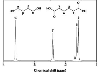
**Fig. A.1.** 1D <sup>1</sup>H NMR spectrum of residues present in water after ageing of unstabilized
