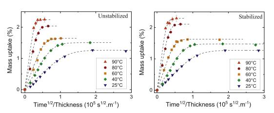
Fig. 2. Mass uptake in immersion at different temperatures, for unstabilized and stabilized TPUs. Corresponding 1D fickian law is plotted in dashed lines.
