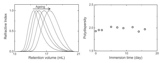
Fig. 6. Chromatograms from initial to 16 days immersion at 80 °C for unstabilized TPU (left) and corresponding Polydispersity (right).
