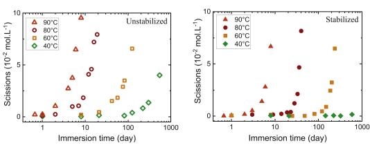
Fig. 9. Effect of temperature on chains scissions kinetics for unstabilized (left) and stabilized (right) TPUs.
