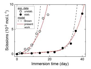
Fig. 13. Comparison of best fit of experimental data obtained with Brown's model and the model developed in the present work (ageing at 80  $^{\circ}$ C).
