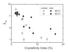
**Fig. 18.** Elongation at break in uniaxial tension as a function of crystallinity index for both TPUs aged in water at 60 and 80  $^{\circ}$ C.
