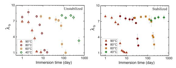
Fig. 10. Elongation at break as a function of immersion time from 40 to 90 °C for unstabilized (left) and stabilized (right) TPUs.
