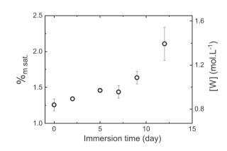
**Fig. 4.** Mass uptake at saturation ( $\%_{m sat.}$ ) and corresponding water concentration [W] as function of immersion time (unstabilized TPU, saturated at 25 °C after ageing at 80 °C followed by drying).
