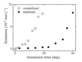
**Fig. 7.** Chains scissions concentration vs. immersion time at 80 °C for unstabilized and stabilized TPUs.
