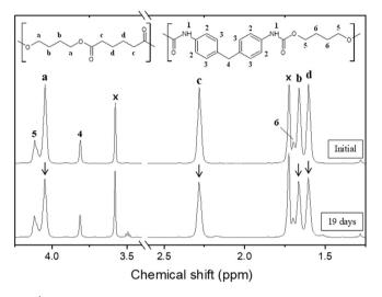
**Fig. 5.** <sup>1</sup>H-NMR spectra of unstabilized TPU, solubilised in THF, in its initial state and after aging in water at 80 °C for 19 days. Peaks are attributed to corresponding protons with letters for adipate soft block, and numbers for urethane hard block. Peaks identified with an x result from solvent response. Arrows indicate peaks change during ageing.
