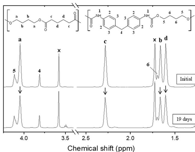
**Fig. 5.**  $^1\text{H-NMR}$  spectra of unstabilized TPU, solubilised in THF, in its initial state and after aging in water at  $80^\circ\text{C}$  for 19 days. Peaks are attributed to corresponding protons with letters for adipate soft block, and numbers for urethane hard block. Peaks identified with an x result from solvent response. Arrows indicate peaks change during ageing.
