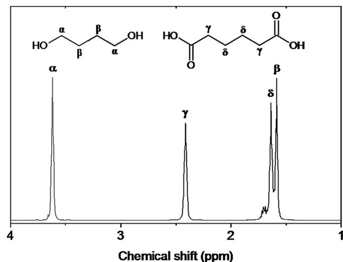
**Fig. A.1.** 1D  $^1H$  NMR spectrum of residues present in water after ageing of unstabilized TPU in water at 80 °C for 42 days, in closed environment. Analysis was performed on  $D_2O$  phase, after solubilisation in a  $CDCl_3 / D_2O$  mixed solvent. Peaks are identified to corresponding protons of adipate hydrolysis products: 1,4-butanediol and adipic acid.
