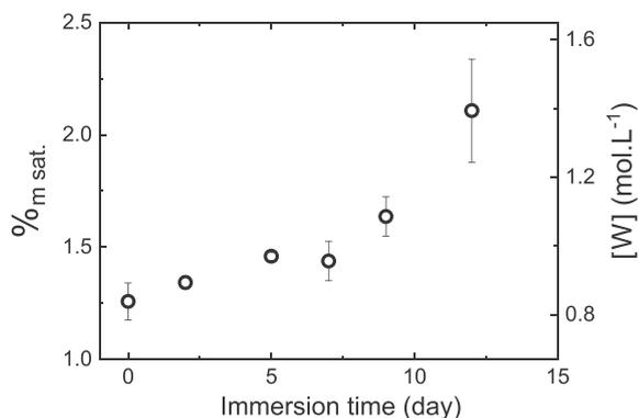
**Fig. 4.** Mass uptake at saturation ( $\%m_{\text{sat}}$ ) and corresponding water concentration  $[W]$  as function of immersion time (unstabilized TPU, saturated at  $25^\circ\text{C}$  after ageing at  $80^\circ\text{C}$  followed by drying).
