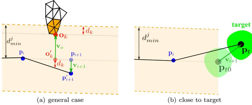
**Fig. 3** Illustration of the correction step in RTIT method: (a) in the general case,  $\mathbf{p}'_{i+1}$  is the modified position of  $\mathbf{p}_{i+1}$  by  $\mathbf{v}_{i+1}$  to avoid the obstacle. For a single risky point  $\mathbf{v}_{i+1} = \mathbf{v}_k$  (b) close to the target,  $\mathbf{p}_{i+1}$  is  $\mathbf{p}_t$ .
