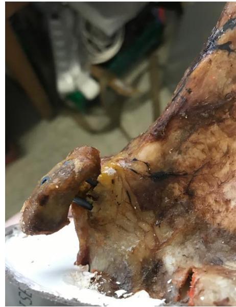
Fig. 4: One example of fixation failure : screws cut-out
