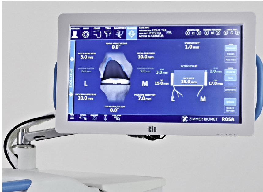
Fig. 1. Following this step, intraoperative planning was performed by each surgeon, using the dedicated software, to determine the ideal resection thickness and angle to obtain a balanced and well-aligned TKA.
