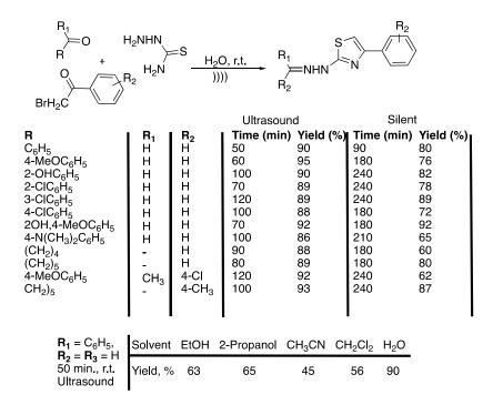
**Scheme 8.** One-pot, three-component, catalyst-free synthesis of N-(4-arylthiazol-2-yl) hydrazones in water under ultrasonic irradiation. The ultrasonic cleaner bath used f = 25 kHz,  $P_{input} = 250 \text{ W}$ , and  $T = 25 ^{\circ}\text{C}$ . Adapted from Zhang et al. [42].
