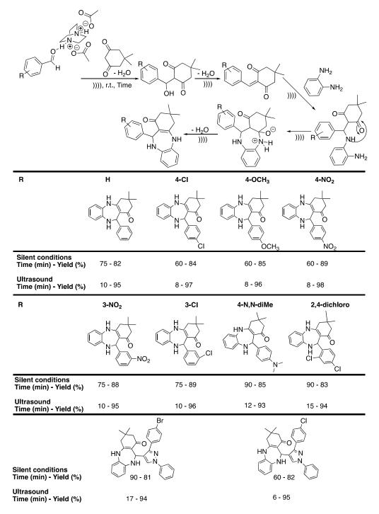
**Scheme 18.** DABCO-triacetate-assisted synthesis of benzodiazepines under ultrasound in solvent-free conditions. Yields are isolated. The ultrasonic bath used f = 45 kHz and  $P_{input} = 305 \text{ W}$ . Adapted from Fekri et al. [99].
