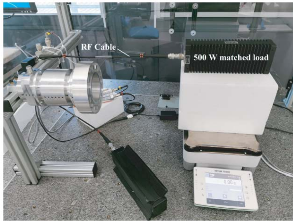
Figure 6. Configuration of the former setup with a RF cable connected to the matched load.
