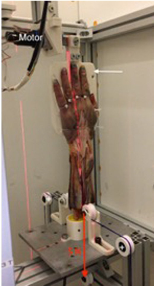
Fig. 2. Test bench. Legend: the asterisk (*) represents the 3D printed base fixed to the reference plane. The crosses (+), the pulleys guiding the cables with 500g masses (red arrow). The white arrow indicates the plate on which are fixed the fingers and the palm with the aid of a clamp. An intermediate piece connects it to the motor.
