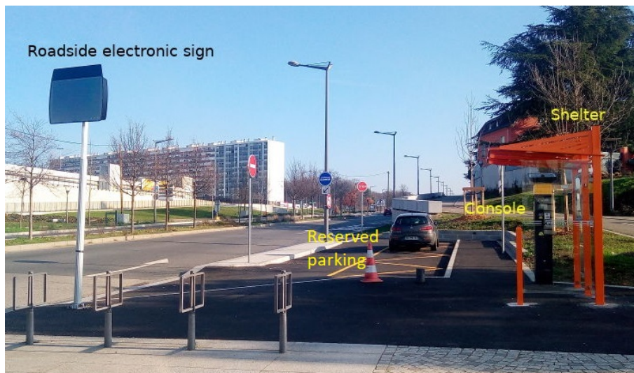
Figure 1: Configuration of a physical meeting point for the “Lane” real-time carpooling service. The orange structure functions like a bus shelter. A passenger notifies potential drivers of their carpooling request using the console, which is then displayed on the roadside electronic sign. A driver can safely embark the passenger in the reserved parking place. Reproduced with permission from Ecov.
