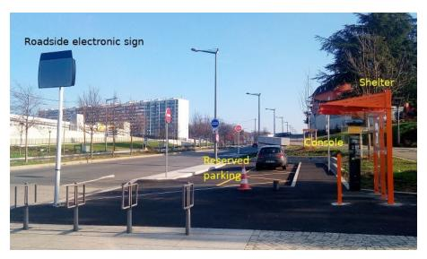
Figure 1: Configuration of a physical meeting point for the "Lane" real-time carpooling service. The orange structure functions like a bus shelter. A passenger notifies potential drivers of their carpooling request using the console, which is then displayed on the roadside electronic sign. A driver can safely embark the passenger in the reserved parking place. Reproduced with permission from Ecov.
