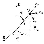
Figure 1: Spherical coordinate system. r: radial coordinate;  $0 \le \theta \le \pi$ : polar or colatitude angle;  $0 \le \phi \le 2\pi$ : azimuthal angle.
