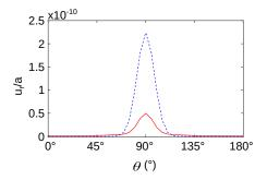
Figure 16: Normal displacement  $u_r(\theta)/a$  at the surface (r = a) of a viscoelastic sphere coated with epoxy. Blue dashed curve: at  $\phi = 0$  and  $t = 4.669 \ \mu$ s. Red solid curve: at  $\phi = \pi/2$  and  $t = 19.14 \ \mu$ s. Source parameter:  $\theta_{\sigma} = 0.1514$ .
