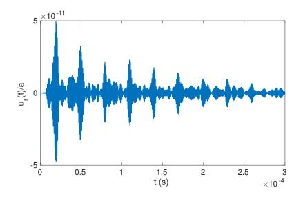
Figure 15: Transient collimating signal  $u_r(t)/a$  at the surface (r = a) of a viscoelastic sphere coated with epoxy at point  $\theta = \pi/2$ ,  $\phi = \pi/2$ . Source parameter:  $\theta_{\sigma} = 0.1514$ .
