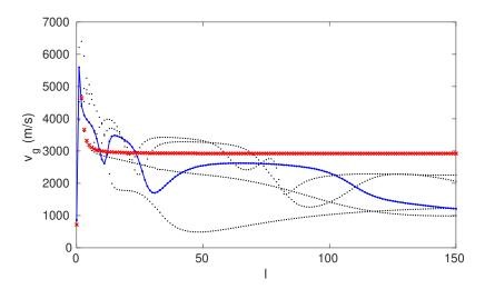
Figure 14: Group velocity of the spheroidal modes of a viscoelastic steel sphere of radius a = 25 mm. Red crosses: Rayleigh mode (n = 1) without coating. Bullets: modes with a 1-mm coating of epoxy (in blue, the quasi-Rayleigh mode).
