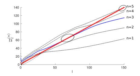
Figure 13: Non-dimensional eigenfrequencies  $\overline{\omega}_l^{(n)}$  of the spheroidal modes of a viscoelastic steel sphere of radius a = 25 mm. Red crosses: Rayleigh mode (n = 1) without coating. Bullets: modes with a 1-mm coating of epoxy (in blue, the quasi-Rayleigh mode).
