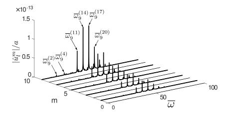
Figure 10: FRF  $|\hat{u}_l^m(\omega)|/a$  at the surface of a viscoelastic sphere (r = a) for l = 9 for the collimating wave  $(\theta_{\sigma} = 0.1514)$ .
