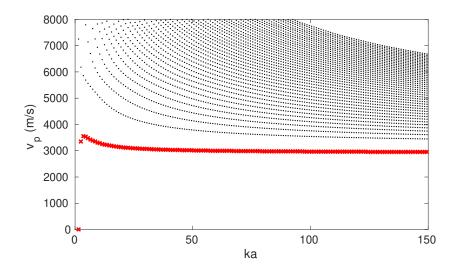
Figure 7: Phase velocity of spheroidal modes for a viscoelastic steel sphere of radius a = 25 mm. Red crosses: Rayleigh fundamental mode (n = 1).
