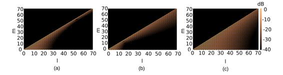
Figure 8: Coefficients  $10 \log_{10}(|\hat{\mathbf{t}}_l^m/\max \hat{\mathbf{t}}_l^m|)$  (dB) of the force applied to obtain (a) a collimating wave ( $\theta_{\sigma} = 0.1514$ ); (b) a focusing wave ( $\theta_{\sigma} = 0.2668$ ); (c) a diverging wave ( $\theta_{\sigma} = 0.0667$ ). These coefficients are computed from the numerical SHT analysis based on Eq. (45) with *l* from 0 to 150, 151 GLQ and 512 FFT points.
