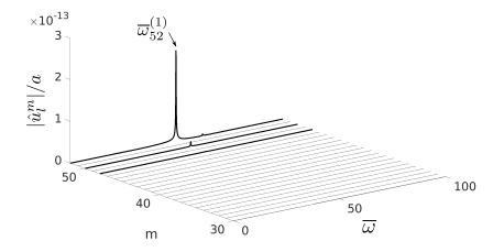
Figure 11: FRF  $|\hat{u}_l^m(\omega)|/a$  at the surface of a viscoelastic sphere (r = a) for l = 52 for the collimating wave  $(\theta_{\sigma} = 0.1514)$ .
