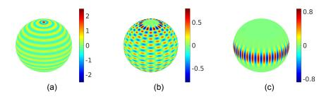
Figure 4: Normal modal displacement (arbitrary unit)  $u_r(r = a, \theta, \phi)$  of the fundamental spheroidal modes l = 30, n = 1 ( $\overline{\omega}_{30}^{(1)} = 29.46$ ) (a) for m = 0; (b) for m = 10; (c) for m = l.
