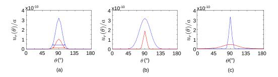
Figure 6: Normal displacement  $u_r(\theta)/a$  at the surface of a viscoelastic sphere (r = a). Blue dashed curve: at  $\phi = 0$  and  $t = 2.289 \ \mu$ s. Red solid curve: at  $\phi = \pi/2$  and  $t = 15.38 \ \mu$ s. (a) Collimating wave  $(\theta_{\sigma} = 0.1514)$ ; (b) Focusing wave  $(\theta_{\sigma} = 0.2668)$ ; (c) Diverging wave  $(\theta_{\sigma} = 0.0667)$ .
