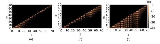
Figure 9: Forced response  $10 \log_{10}(|\hat{u}_l^m/\max \hat{u}_l^m|)$  (dB) at the surface of a viscoelastic sphere (r = a) and at the centre frequency  $(\overline{\omega} = 49.46)$  for (a) a collimating wave  $(\theta_{\sigma} = 0.1514)$ ; (b) a focusing wave  $(\theta_{\sigma} = 0.2668)$ ; (c) a diverging wave  $(\theta_{\sigma} = 0.0667)$ .
