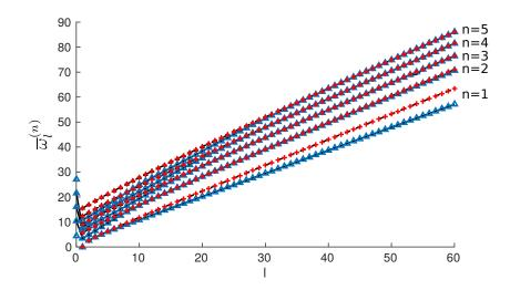
Figure 2: Non-dimensional eigenfrequencies  $\overline{\omega}_l^{(n)}$  of a surface-free sphere made of steel. Solid and dashed blacked lines: results of Eringen and Şuhubi [19] for spheroidal and torsional modes. Blue triangles: numerical results for spheroidal modes. Red crosses: numerical results for torsional modes.
