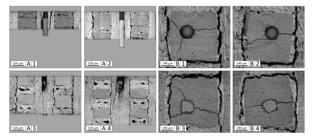
**Figure 6.** Bundle push-out tests. A: Postmortem sectional observations on several thicknesses. B: Postmortem surface observations.
