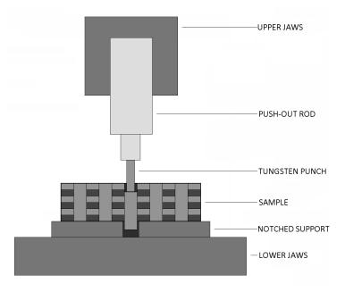
Figure 3. Room temperature push-out experiemtnal setup.
