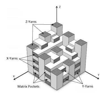
Figure 1. Structure and constituents of the 3D C/C.
