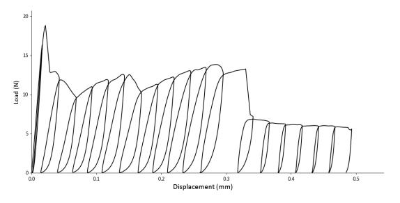
Figure 7. Cycled bundle push-out test measurement.
