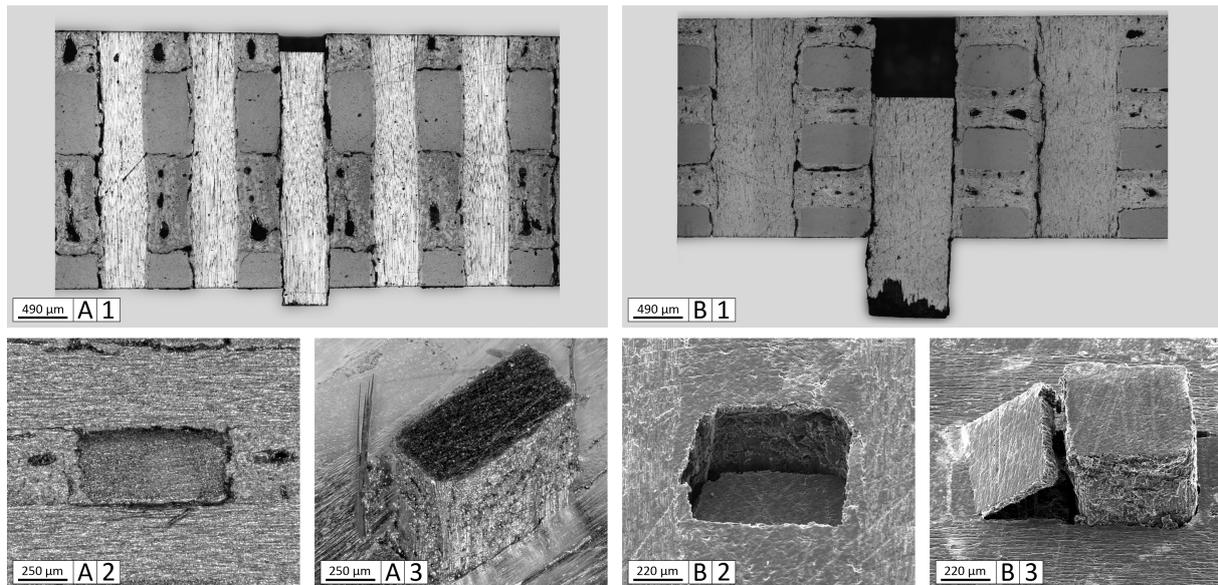
**Figure 4.** Postmortem sectional (1) and top (2) and bottom (3) surface observations for X/Y (A) and Z (B) yarn push-outs.
