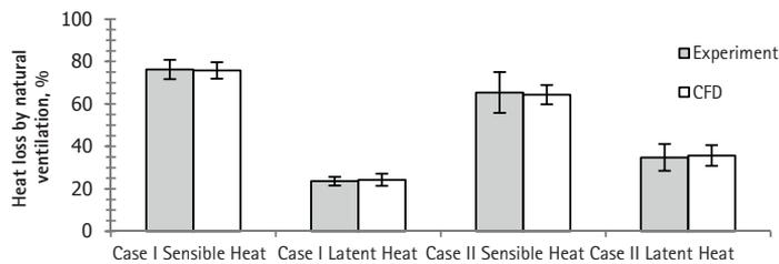
Fig. 3: Experimental and predicted sensible and latent heat losses with the operating conditions for Cases I and II - 100 % as described in Table 1
