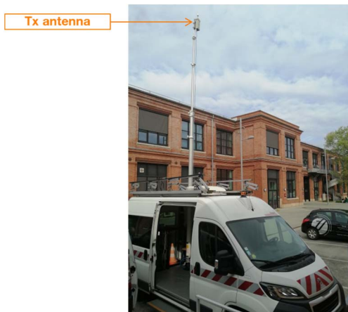
Fig. 4. Tx antenna on the roof of the measurements truck
