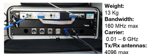
Fig. 1. Portable wideband channel sounder
