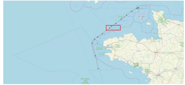
Fig. 3. Anomaly due to extreme weather condition. Because of a strong wind blew from the opposite direction, this vessel slowed down (in the red zone). Some similar cases were detected at the same night.
