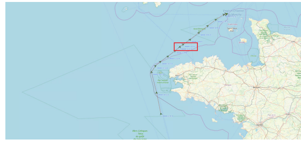
Fig. 3. Anomaly due to extreme weather condition. Because of a strong wind blew from the opposite direction, this vessel slowed down (in the red zone). Some similar cases were detected at the same night.
