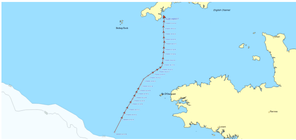
Fig. 8. An AIS track flagged as abnormal by the original model but considered as normal by the new model. This track is actually normal. However, in the original training set, there are not many tracks of this type (because they are outside of the coverage zone of the terrestrial AIS station), hence it was flagged as abnormal. The coverage area of the new dataset is better, GeoTrackNet then succeeded to tag this track as normal.
