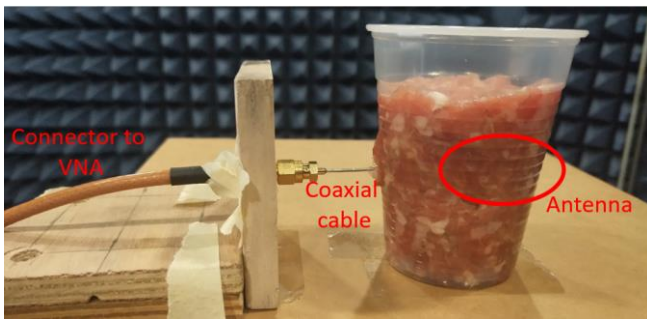
Fig 7. [a] fabricated antenna comparing with one euro cent [b] complete antenna with coaxial cable and superstrate [c] antenna embedded into minced pork
