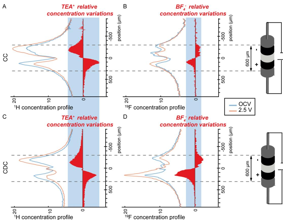
Figure 2. (A,C)  $^1\text{H}$  and (B,D)  $^{19}\text{F}$  1D concentration profiles of a supercapacitor made of a CC (A,B) and CDC (C,D), during OCV before charging and at 2.5 V. The profiles of the concentration changes on charge (between 2.5 V and OCV) are displayed on the right of the profiles as filled red curves.
