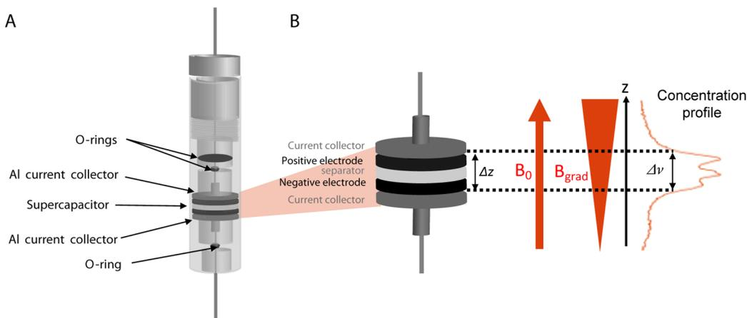
Figure 1. (A) *In situ* electrochemical cell containing the supercapacitor (5 mm diameter, 600  $\mu\text{m}$  thickness once assembled). (B) Vertical  $^{19}\text{F}$  spin density profile obtained from the  $^{19}\text{F}$  NMR signal of the electrolyte.
