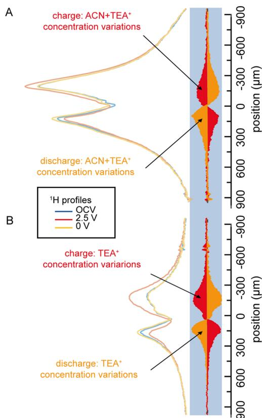
**Figure 4.** Charge/discharge 1D TEA<sup>+</sup> concentration profiles (left) during OCV, at 2.5 and 0 V, and the corresponding changes on the same scale (right: red for charge and orange for discharge) observed for a supercapacitor made with CC with (A) non-deuterated and (B) deuterated acetonitrile.
