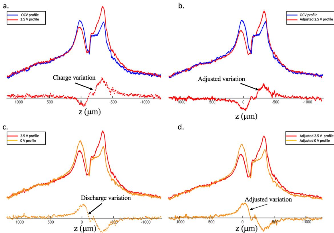
Figure S6.  $^1\text{H}$  concentration profiles of a supercapacitor under open circuit (blue), at 2.5 V (red) and at 0 V (yellow) after discharge. Concentration variation profiles for charge (a. and b.) and discharge (c. and d.), with no scaling (left) and scaling (right).
