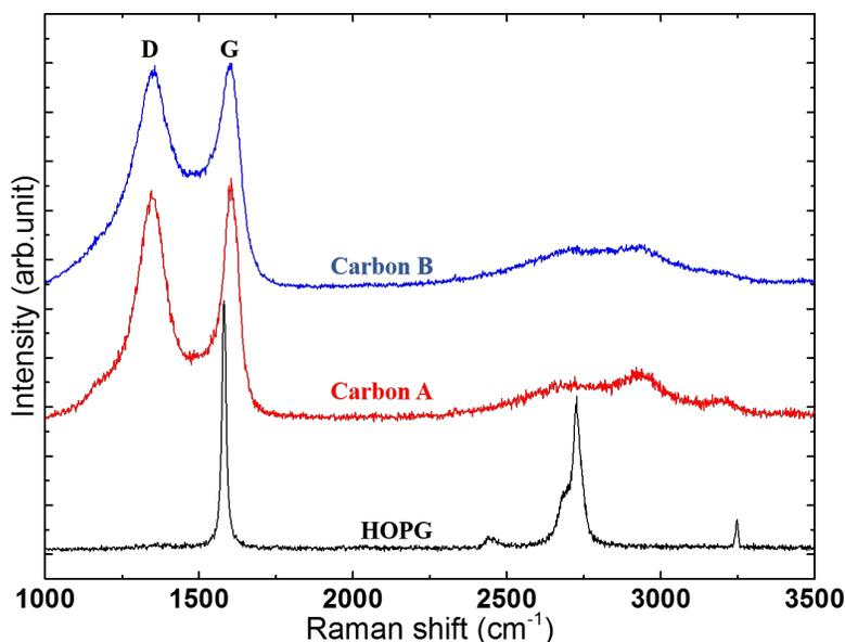
Figure S3. Raman spectra obtained for CC (carbon A - red) and CDC (carbon B - blue), using a laser energy of  $2.41\text{eV}$  ( $514.5\text{nm}$ ). The spectrum of HOPG (Highly oriented pyrolytic graphite) is displayed as a reference in black.
