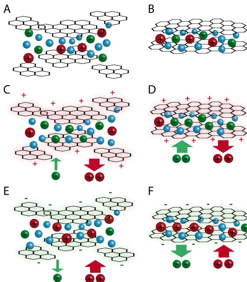
**Figure 3.** (A,B) Open-circuit contents of the pores for (left) CC and (right) CDC. The CC has both small and large nanopores, whereas the CDC has a majority of small nanopores, displayed here as slit-shaped spaces between carbon layers. Charge mechanism in (C,D) for the positive electrode and (E,F) for the green negative electrode, showing the observed anion and cation flux in the carbon electrode upon charging.
