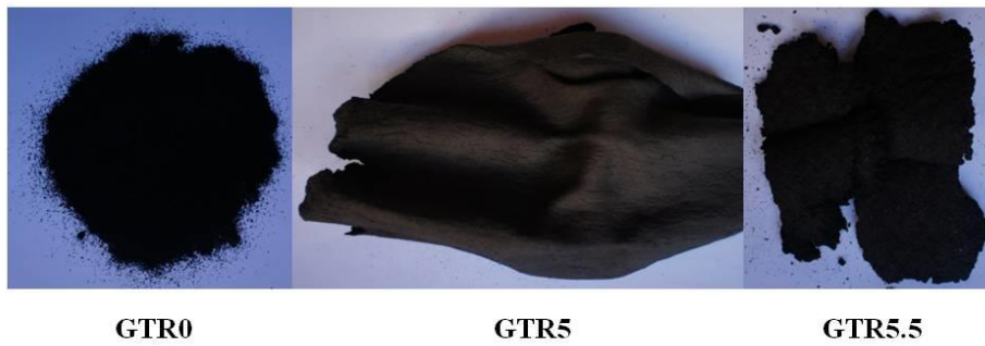
Figure 12 - Photos of GTR0, GTR5 and GTR5.5 after remixing in a two roll mill.
