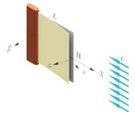
Figure 1: Two-dimensional inverted flag in axial flow: free at the upstream and clamped at the downstream end. The flag is assumed to be infinitely wide (i.e.  $H/L \rightarrow \infty$ ); hence, the fluid flow surrounding the flag is treated as two-dimensional.
