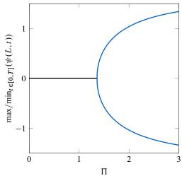
Figure 11: Bifurcation diagram of an inverted flag subjected to steady-fluid forces showing the leading edge rotation angle versus dimensionless flow velocity. [---] Undeflected stable equilibrium and [---] deflected static equilibrium solutions corresponding to buckling of the inverted flag to either side. No secondary bifurcation (dynamic or static) materializes. Colour scheme as in figure 6.
