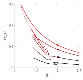
Figure 17: Reduced frequency of the asymmetric flapping motion as a function of the dimensionless flow velocity  $\Pi$  for  $\psi_0 = 0.2$  and different mass ratios:  $[\blacktriangle] \mu = 0.1$ ,  $[\blacksquare] \mu = 0.5$ ,  $[\bullet] \mu = 2.0$ , and  $[\bullet] \mu = 5.0$ .  $[\bullet \bullet \bullet]$  Unstable and  $[\bullet \bullet]$  stable periodic solutions.
