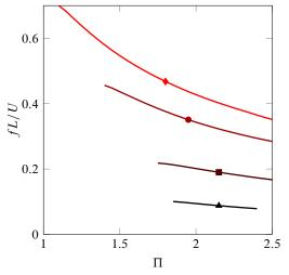
Figure 13: Sensitivity of the large-amplitude flapping reduced frequency to the dimensionless flow velocity  $\Pi$  for inverted flags of different mass ratios: [ $\blacktriangle$ ]  $\mu = 0.1$ ; [ $\blacksquare$ ]  $\mu = 0.5$ ; [ $\bullet$ ]  $\mu = 2.0$ ; and [ $\bullet$ ]  $\mu = 5.0$ .
