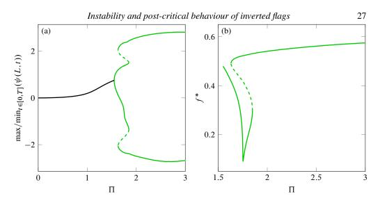
Figure 15: Nonlinear response of a two-dimensional inverted flag with  $\mu = 1.0$  and  $\psi_0 = 0.1$ . (a) Bifurcation diagram indicating the minimum and maximum values of the leading edge rotation over a cycle of steady-state oscillation of period  $T^*$ : [—] Stable static solution; [---] unstable and [—] stable periodic solution (asymmetric oscillations). (b) Dimensionless frequency  $f^*$  versus dimensionless flow velocity  $\Pi$ .
