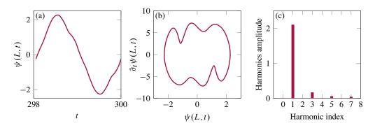
Figure 9: Response of the inverted flag with  $\mu = 1.0$  at  $\Pi = 1.65$ , displaying a periodic motion around the undeflected equilibrium; (a) time history, (b) phase-plane portrait, and (c) the frequency content of the response, obtained from FFT. Colour scheme as in figure 6.
