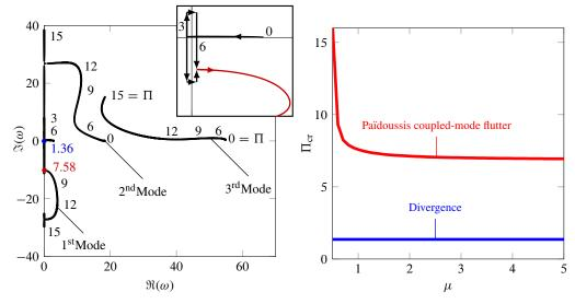
Figure 4: Argand diagram for an inverted flag with  $\mu = 1.0$ , showing the evolution of the first three modes with the dimensionless flow velocity  $\Pi$ .
