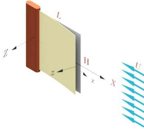
Figure 1: Two-dimensional inverted flag in axial flow: free at the upstream and clamped at the downstream end. The flag is assumed to be infinitely wide (i.e.  $H/L \rightarrow \infty$ ); hence, the fluid flow surrounding the flag is treated as two-dimensional.
