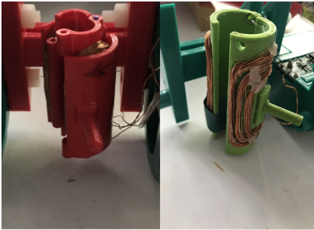
Figure 2. SHS clampable coils dedicated to the low-field NMR (8 mT) device. Their resonant frequency was tuned closed to 336 kHz (corresponding to the ^1\text{H} Larmor frequency at 8 mT). Right figure represents the SHS2 clampable coil and left figure the SHS6. The supporting structure has been realized by 3D printing.
