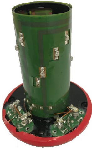
Figure 4. Quadrature SHS4 serial coil dedicated to ^1H 3 T MRI (80 mm length and 42 mm internal diameter). The coils are realized on a same flexible printed circuit board including the pads to welcome the segmentation capacitors. Two tuning–matching PCB, for respectively 0 and 90° driving, are inserted on the lower part of the coil.
