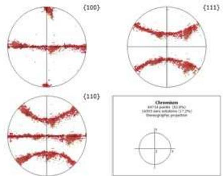
Figure 2 - Typical EBSD orientation maps and associated stereographic pole figures of the first generation 5-10 $\mu$ m-thick Cr-coated Zircaloy-4 (sheet substrate), obtained with different PVD deposition parameters
