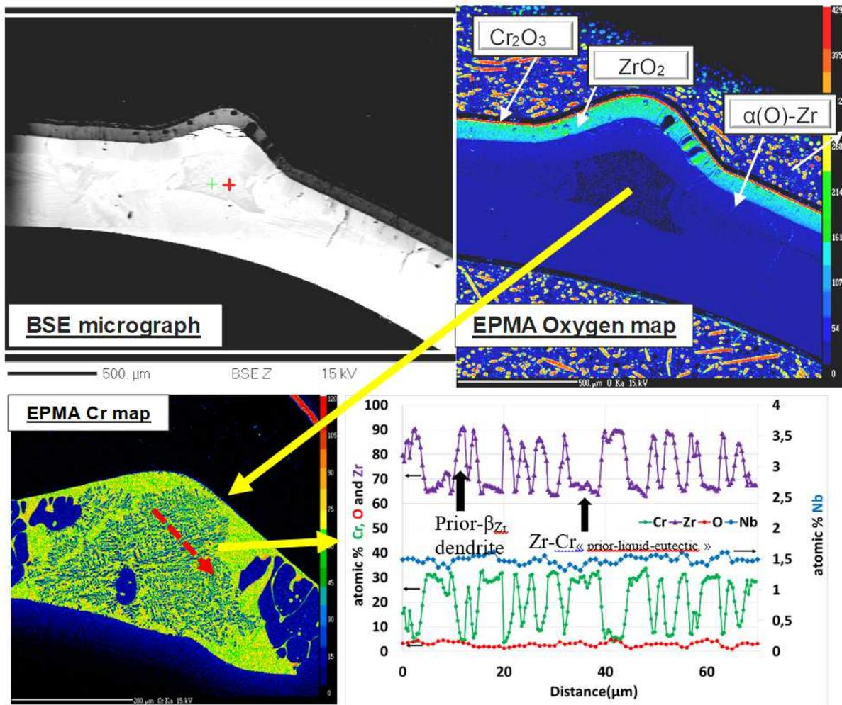
Figure 17 - EPMA chemical element mapping and quantitative profiles obtained at the vicinity of a protruding blister in a Cr-coated M5<sub>Framatome</sub> cladding segment one-sided steam oxidized for 100s at  $\sim 1400\text{-}1450^\circ\text{C}$  and water quenched down to room temperature
