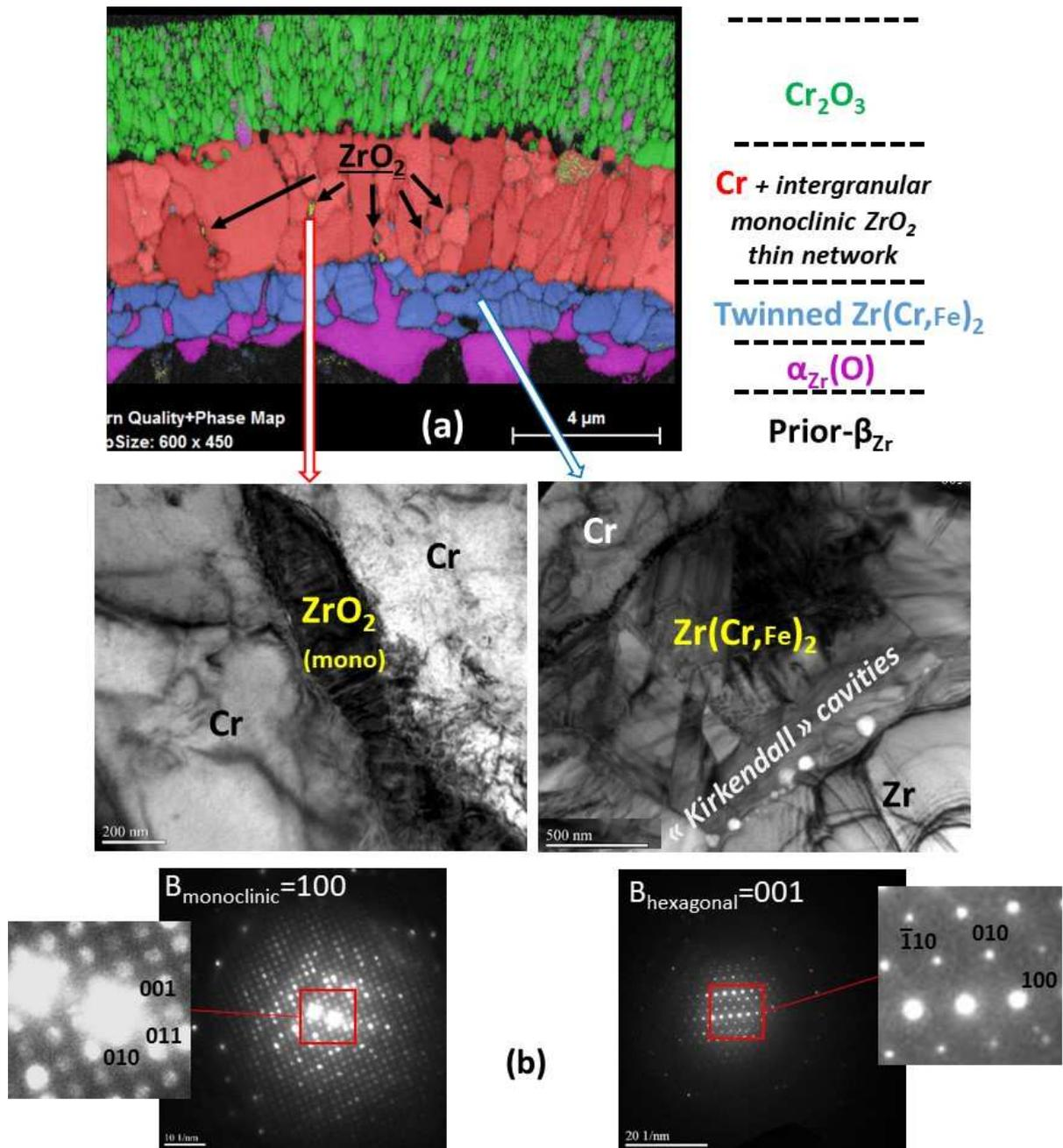
Figure 7 - PQ typical microstructure of a 5-10 $\mu\text{m}$ -thick Cr-coated Zircaloy-4 sheet sample from the first generation after steam oxidation for 1400s at 1200 $^\circ\text{C}$  (transition stage):
