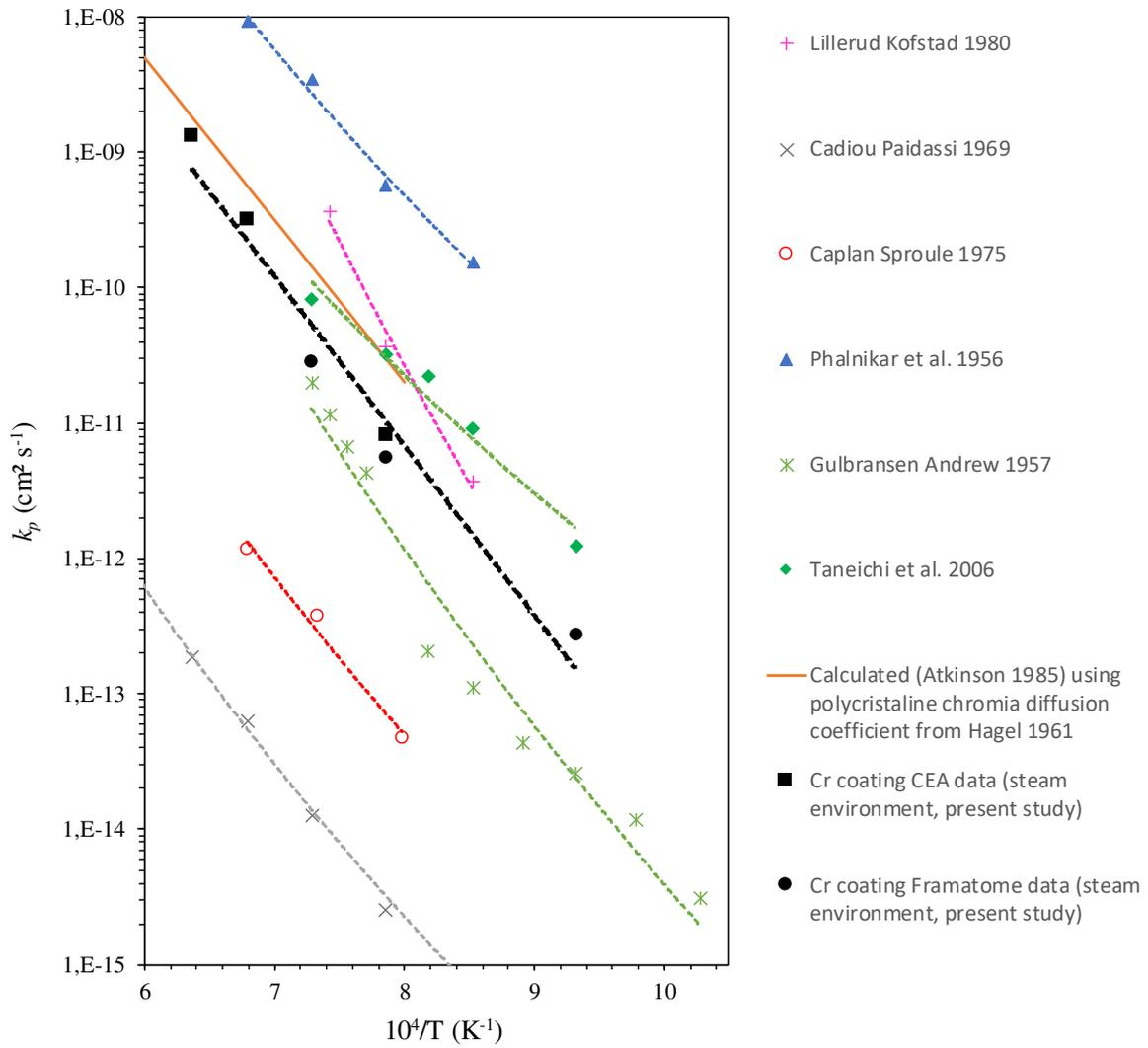
Figure 3 - Arrhenius plot of the rate constant of the parabolic law describing the growth of  $\text{Cr}_2\text{O}_3$  upon HT oxidation, reported in the literature for pure chromium (oxidized in air or oxygen) [41]-[48] (replotted from [49]) and from the present study for Cr-coatings (steam oxidation, short oxidation times)
