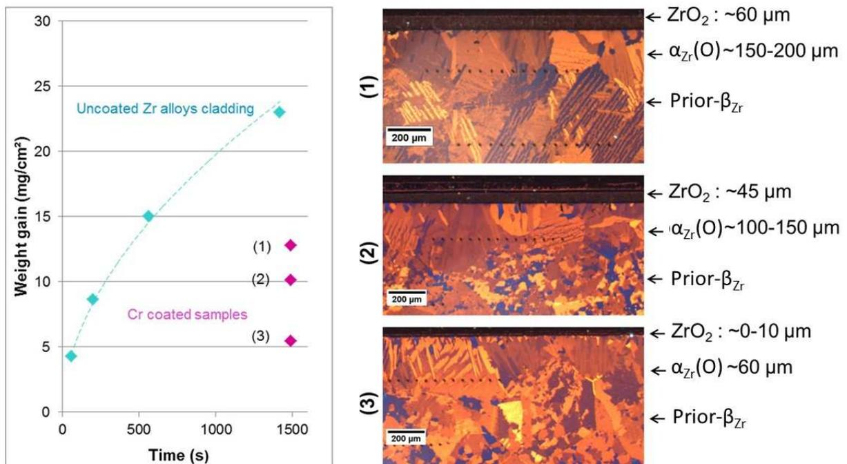
Figure 10 - Comparison of the weight gains of uncoated and 6-8μm-thick Cr-coated Zr alloys claddings after steam oxidation at 1200°C and corresponding PQ optical micrographs (polarized light):
