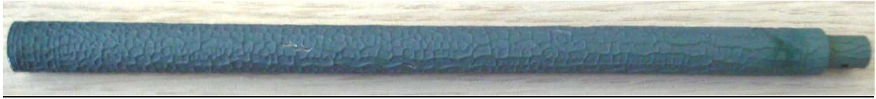
Figure 16 - Typical PQ aspect of a 12-15 $\mu\text{m}$  thick Cr-coated M5<sub>Framatome</sub> cladding sample after HT oxidation for 100s at 1400°C followed by direct water quenching
