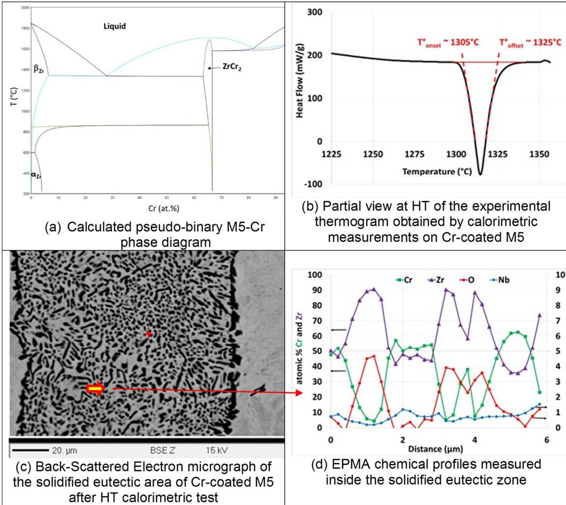
Figure 15 - Calculated pseudo-binary  $M5_{Framatome}-Cr$  phase diagram, partial thermogram from calorimetric measurements, associated microstructures and chemical profiles, underlying the M5-Cr eutectic reaction at temperatures above  $1300^{\circ}C$
