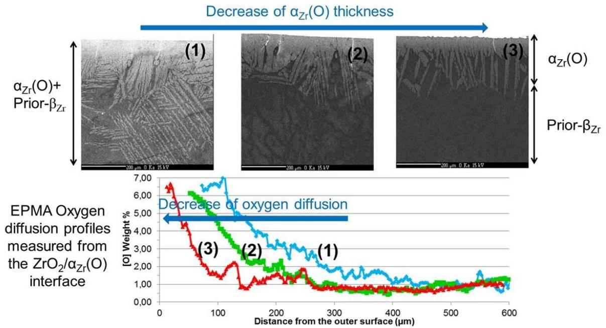
Figure 11 - PQ SEM-BSE micrographs and oxygen concentration profiles (from EPMA measurements) within the inner prior- $\beta_{Zr}$  layer of uncoated and 6-8 $\mu\text{m}$ -thick Cr-coated Zr1Nb(O) alloy steam oxidized for 1500s at 1200°C: (1) as-deposited, (2) pre-annealed 2h at 700°C, (3) pre-annealed 2h at 800°C materials
