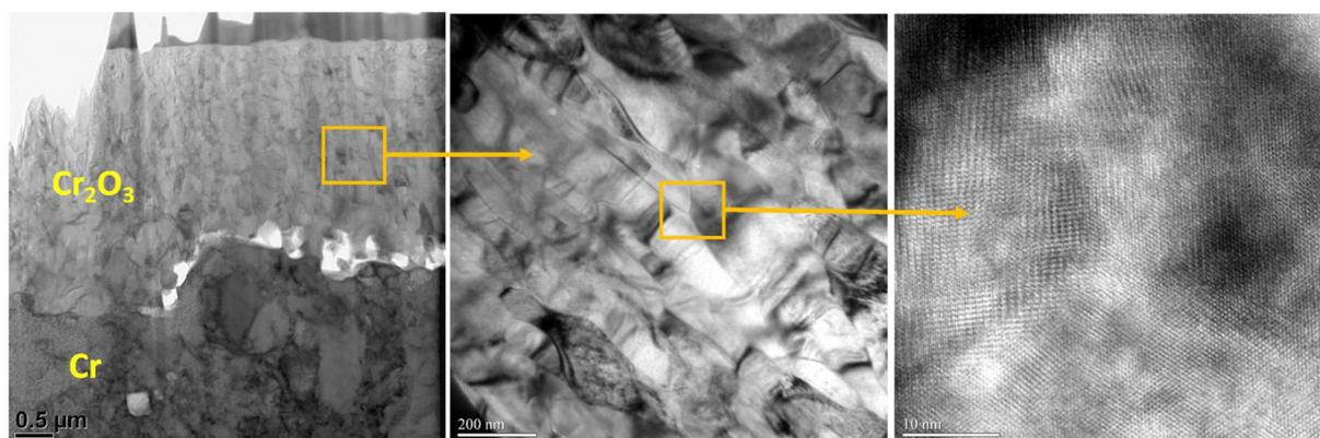
(a) Overall view of Cr<sub>2</sub>O<sub>3</sub>/Cr outer scales (low magnification)
