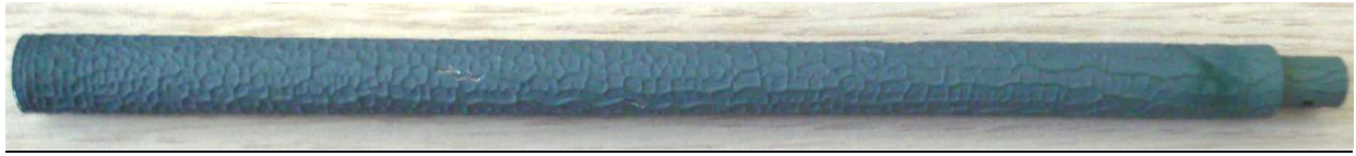
Figure 16 - Typical PQ aspect of a 12-15 \mu\text{m} thick Cr-coated M5 Framatome cladding sample after HT oxidation for 100s at 1400°C followed by direct water quenching
