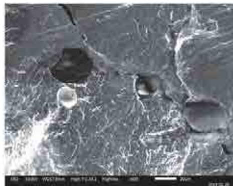
(d) Crack propagation through pores (SEM - secondary electrons)
