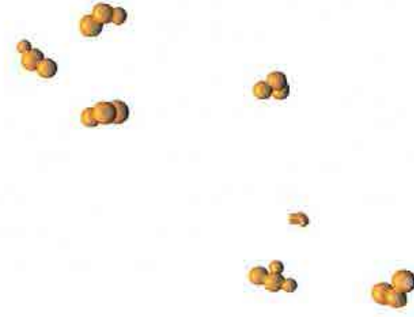
Figure 16. Merged pores inducing low sphericities (adhesive B, high temperature curing).
