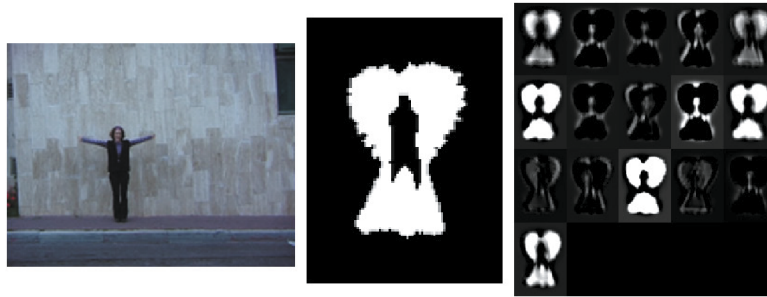
Fig. 12. (Color online) Sample from Weizmann dataset: (left) Wave2, (Middle) extracted BSTM, (right) activations of the first convolutional layer.
