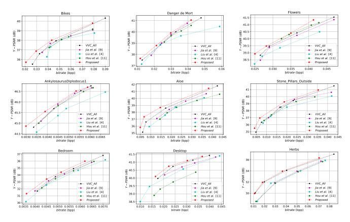
Fig. 4. RD curves of the five considered solutions for the 9 LF images using four QP values.
