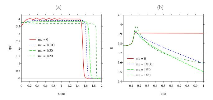
Figure 11: Variable boundary conditions (104)-(105): influence of the dissipation parameter  $\mu$  in (73e). (a) snapshots of  $\varepsilon$  at t=1 s. (b) time evolution of the discrete energy (87).
