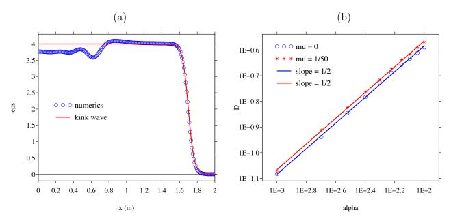
Figure 12: Variable boundary conditions (104)-(105): influence of the regularization parameter  $\alpha$  on the shape of the front. (a): comparaison between the numerical solution and the kink wave (27), at t = 0.6 s and for  $\alpha = 5.10^{-3}$ . (b) log-log plot of D vs  $\alpha$ , for two values of  $\mu$ , and linear regression with slopes 1/2.
