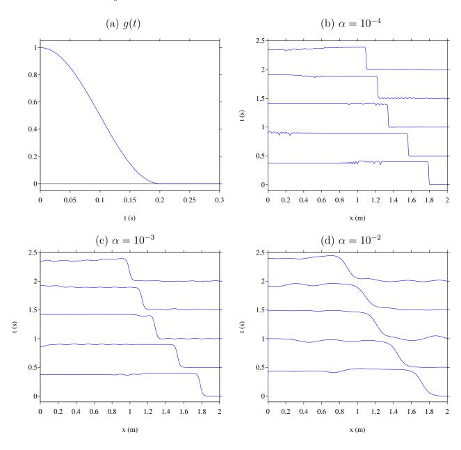
Figure 10: Variable boundary conditions. (a): forcing g(t) in (104)-(105), with  $f_c = 5$  Hz. (b,c,d): snapshots of  $\varepsilon$  at successive instants and for various values of the regularization parameter  $\alpha$ .
