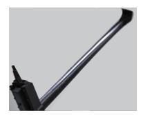
Figure 1: Dynamic deployment of a bistable tape spring. From a coiled configuration to a deployed straight one, from left to right.
