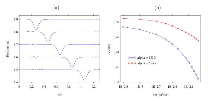
Figure 13: Variable boundary conditions (104)-(105): influence of the dissipation parameter  $\mu$  and of the regularization parameter  $\alpha$  on the speed V of the front. (a) time evolution of p at the receivers. (b) plot of V vs  $\mu$ , for two values of  $\alpha$ .
