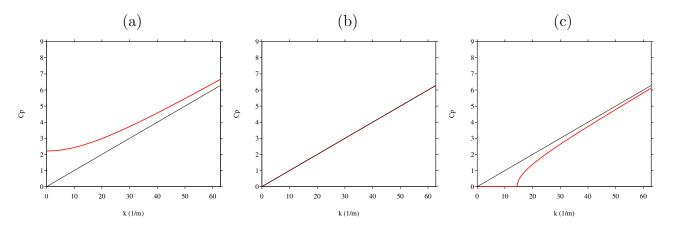
Figure 3: Master Lagrangian phase velocity (20), for three values of  $\bar{\varepsilon}$ , leading to:  $W^{''} > 0$  (a),  $W^{''} = 0$  (b), and  $W^{''} < 0$  (c). The line through the origin is the asymptote  $\sqrt{\alpha/\rho} k$ .
