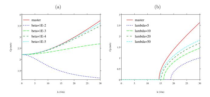
Figure 7: Phase velocities of the master wave  $c_p$  (20) and of the slow wave  $c_p^-$ . (a):  $W^{''} > 0$ ,  $\lambda = 100$  and various values of  $\beta$ . (b):  $W^{''} < 0$ ,  $\beta = 10^{-3}$  and various values of  $\lambda$ .
