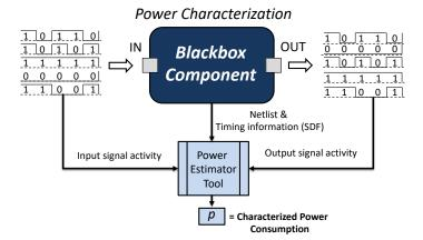
Fig. 3. Detail of the Power Characterization Branch
