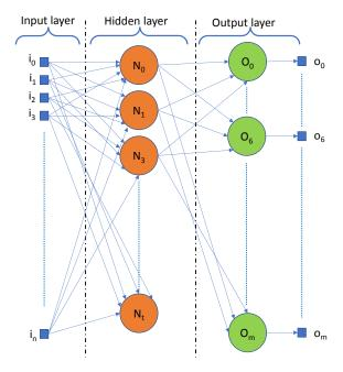
Fig. 1. Multi-Layer Perceptron (MLP) Architecture
