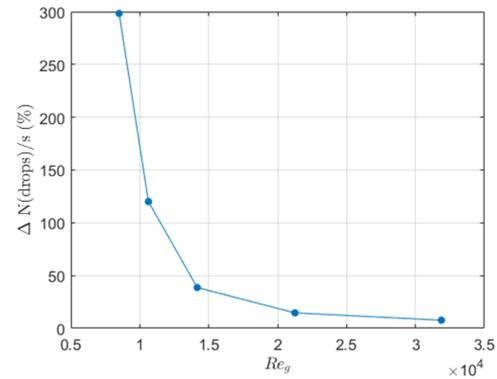
**Figure 7.** Percent difference in the area of the image covered by droplets for the cases with and without electric charge. The charged spray produces a larger volume of droplets (starting from the same volume of liquid), but the difference decreases at high  $Re_g$ .
