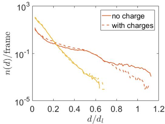
**Figure 6.** Histogram of the droplet size, normalized by the number of frames, in the shadowgraph movies, for  $Re_g = 10, 600$  (red) and  $Re_g = 10, 600$  (yellow) with and without an applied electric field.
